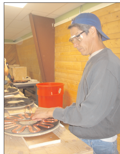
Mille Lacs Band member Patrick Losh is wiring the armature, one of the first stations of assembly at the manufacturing plant.
