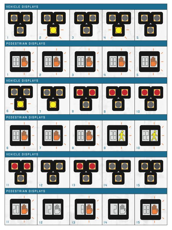
**1.** The vehicle indication remains dark when the pedestrian crossing is not in use. The raised Don't Walk hand symbol remains on during this timing interval. (Note: The number in the lower left corner of the signal display indicates the order in which the signal sequence will occur.)
